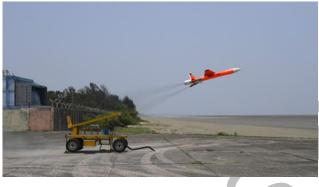
Two demonstrator vehicles of Abhyas cleared all the evaluation parameters like 5 km flying altitude, vehicle speed of 0.5 mach (half the speed of sound), endurance of 30 minutes etc.
