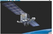
Named Rukmini, the satellite carries payloads in UHF, C-band and Ku-band, and helps the Navy to have a secure, real time communication link between its land establishments, surface ships, submarines and aircraft. The satellite was injected into a geosynchronous transfer orbit (GTO) of 249 km perigee (nearest point to earth), 35,929 km apogee (farthest point to earth) and an inclination of 3.5 degree with respect to the equator.
